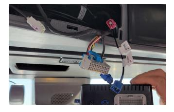
Route FLC5.x cable to SDP5.5 mounting location in center-right of overhead.
