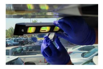
Ensuring that notch B is lined up and when it is level, begin pressing from the top of the bracket onto the window.
