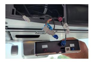
• If the SDP5.5 is already installed, simply plug the antenna cables (blue and pink connectors) into the SDP5.5 sockets (blue and pink sockets).
