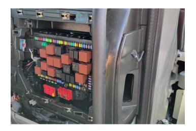
• Locate RS232 connector and bring it out near the passenger door vent.
