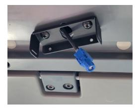
Take the DFC bracket and bring blue connector through the hole in the overhead and bracket. Mount bracket with included screw/nuts as pictured.
