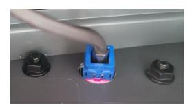
Plug the blue connector into the DFC and with the black Allen bolts attach the DFC to the DFC bracket to hand tight and install the DFC cover.
